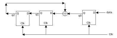
data:100110000 (1 first) is supplied to the "data" terminal in nine clock cycles. After that the value of  $q_2q_1q_0$  are: (A)000 (B) 001 (C) 010 (D) 101
